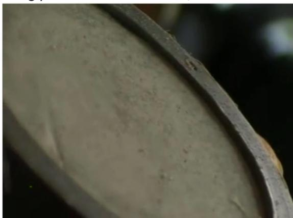
Remove the part of the protective ring that extends beyond the alabaster surface, using a lathe, a grinding machine, or half-round and flat files with decreasing coarseness, followed by sanding with coarse sandpaper. Illustrations are shown in the video (FacingPocisType1\_2017-07-01.mp4).
